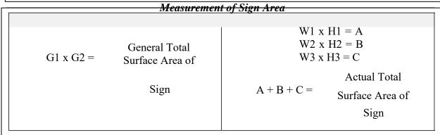
Figure 20.1 – Measurement of Sign Area
