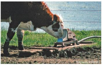
The steer pushes a piston with its nose to power the pump.
