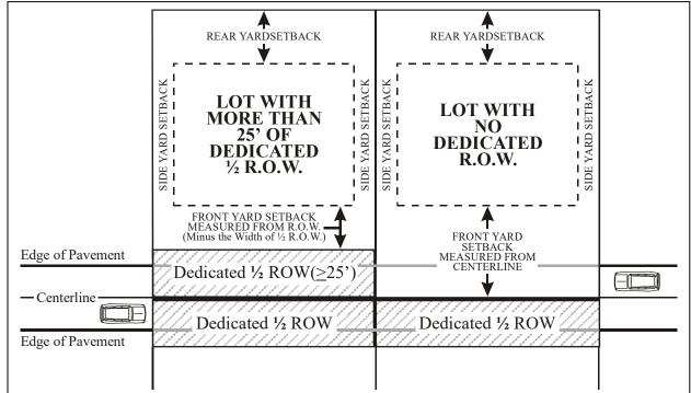
Figure 25.1 - Determining Setbacks from Property Lines
