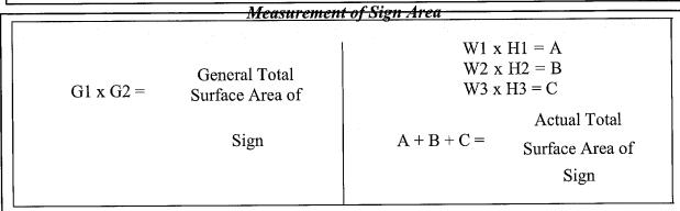
Figure 20.1 – Measurement of Sign Area
