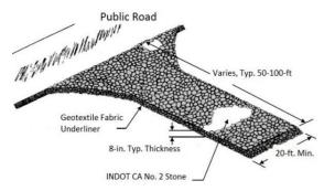
Standard detail of a construction entrance. Be sure to follow the specifications required on the construction drawing. If a construction entrance is not shown, work with your local community contact to ensure an adequate construction entrance is installed.
