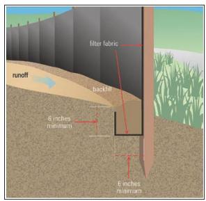
Install silt fence prior to land disturbing activities. Silt fencing should be installed 6 inches deep, at a minimum. Make sure wooden stakes are on the downstream side of the flow.
